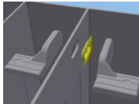
intercell connection (through the partition)
