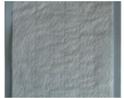
special separator with fleece layer
