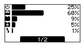
In statistics mode, horizontal bars display the frequency of the following device operating statuses:
